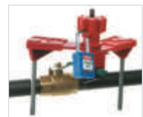
Use two blocking arms to lockout 3-, 4- or 5-way valves, or to lock valves in the throttled position for operational control
